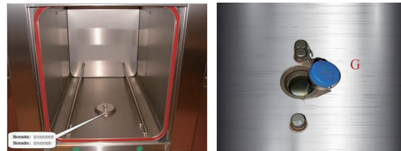
Figure 2 Reference measurement point G, sterilizing chamber exhaust port
